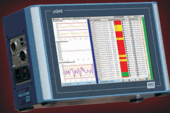
Standard device for the monitoring of one or two welding torches
